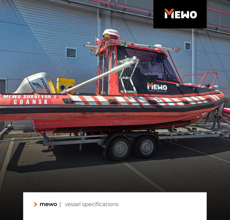
The mobile motorboat designed for costal geophysical surveys and small service works. The unit is equipped with side mounted pool. The workboat can be easily transported by road and launched at the marina.
